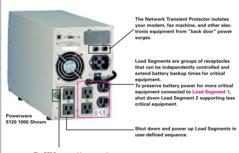
The REPO port enables you to shut down the UPS and connected equipment from a remote location in an emergency.
